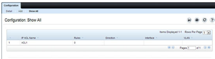
Figure 20-3. View IPv4 ACLs
